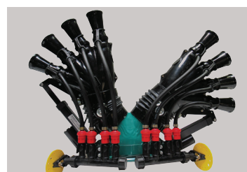
OPTION - Electro cylinders with control box operated from tractor seat (inner spray heads)
